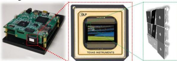
Figure 5 Example of a commercial DMD controller (left, Texas Instruments), a DMD (middle, Texas Instruments) and the three-state positioning of micromirrors ( $+12^\circ$  light grey,  $-12^\circ$  black,  $0^\circ$  dark grey; right).
